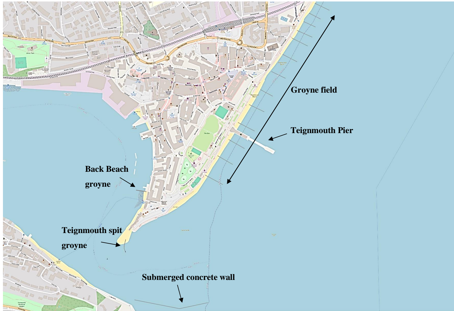
Figure 3-2. Teignmouth coastline featuring various engineered structures. Seawalls extending along the entire frontage of Teignmouth seafront beach, Teignmouth Back Beach and Shaldon Beach.
