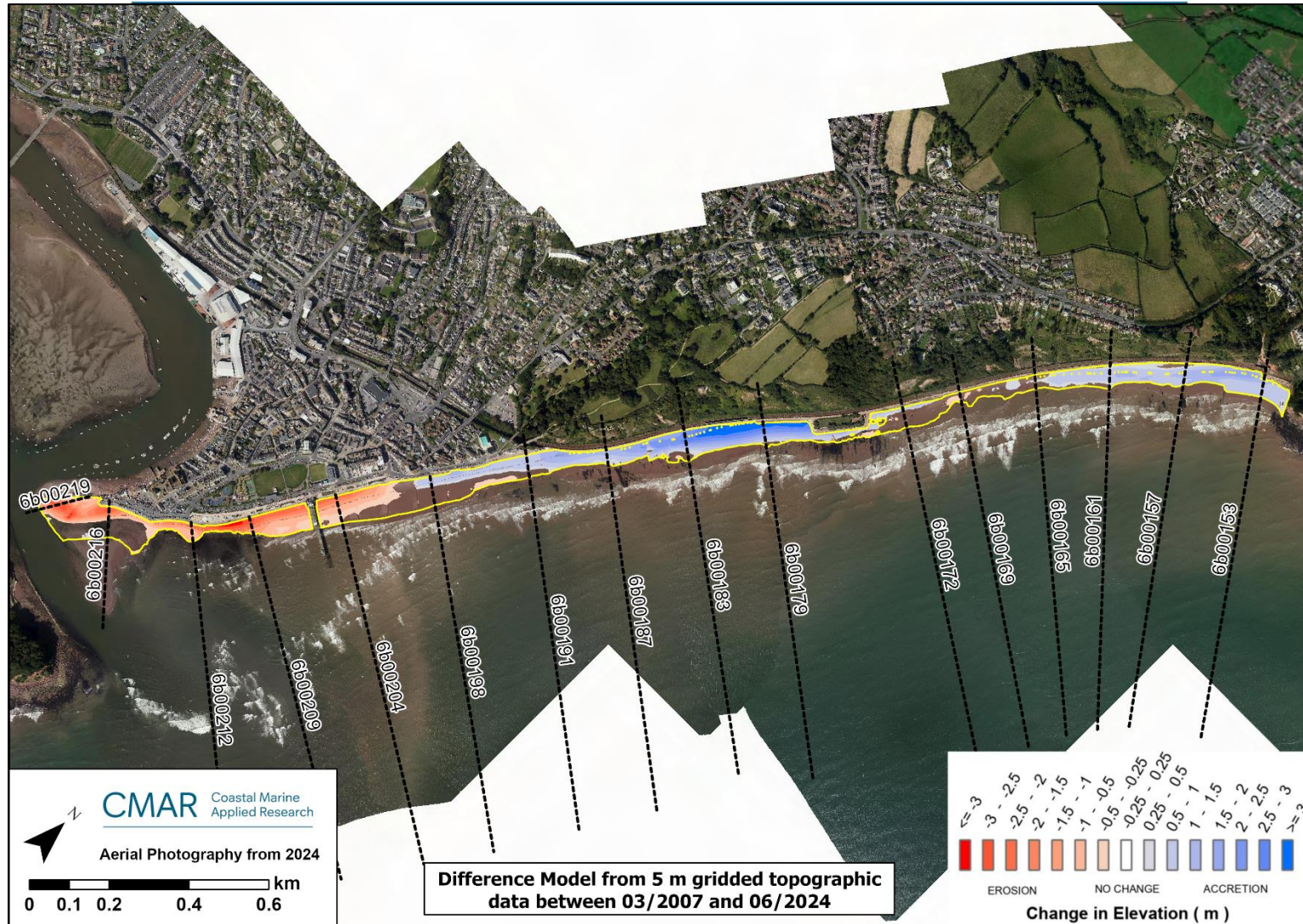
Figure 4-7. Net morphological response for the period 2007–2024 across all of Teignmouth Seafront Beach (Full Extent) from gridded topographic data. Red colour indicates net loss of material and blue colour indicates net gain of material.
