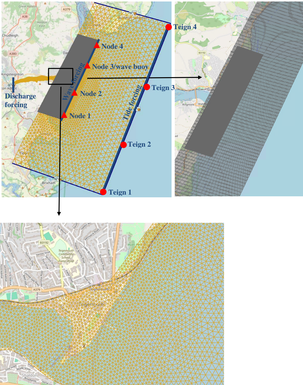
Figure C-2. Model grid showing combined D-FLOW flexible mesh (orange) and two meshes from the D-WAVE module (grey). Upper left panel: overview of all the model grids, forcing boundaries (blue lines), and wave (red triangles) and tide (red circles) forcing nodes. Upper right panel: two grids used in the wave model. Lower panel:
