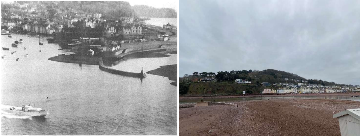
Figure 2.1 Photos showing differences in sand accumulation around The Point breakwater, left: photo from c 1963-4 (Binnes, 2024), and right: Teignmouth BMP site visit photo from 2024.
