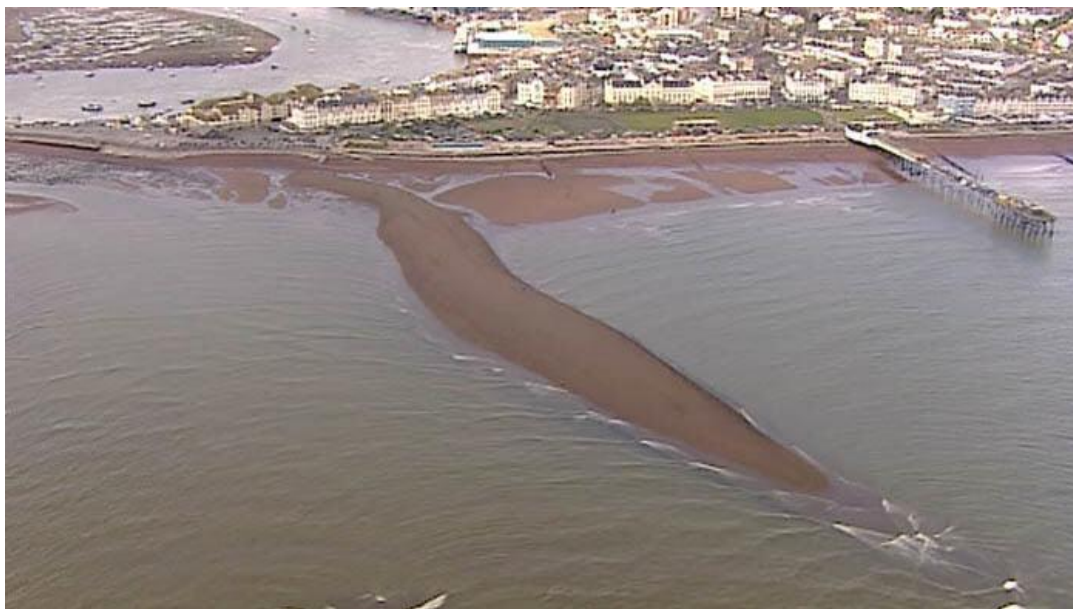
Figure 3-6. The Inner Pole of Teignmouth ebb-tidal delta during a shore-attached phase in 2001. As the Inner Pole migrates to the shore it delivers a significant supply of sand to the beach adjacent to Teignmouth Lighthouse (New Forest District Council, 2017).
